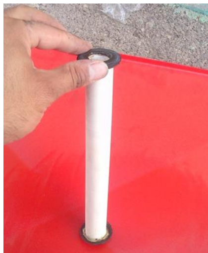
Figure 2: Nanofilter made of carbon-nanotubes.
